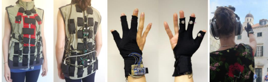
Fig. 3. Mixed reality cues and affordances can be provided through haptic user interfaces: (a) the vest; (b) the glove; and (c) audio-haptic exploration, in which an MRUE user points at a POI with the haptic glove and listens to the associated audio description.
