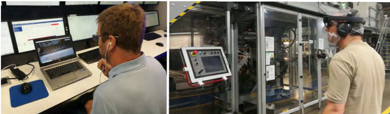
Fig. 1. Facility for production. (left) An expert in the control center dispatching (right) a worker on the shop floor, wearing a HoloLens, to fix machine downtime problems.
