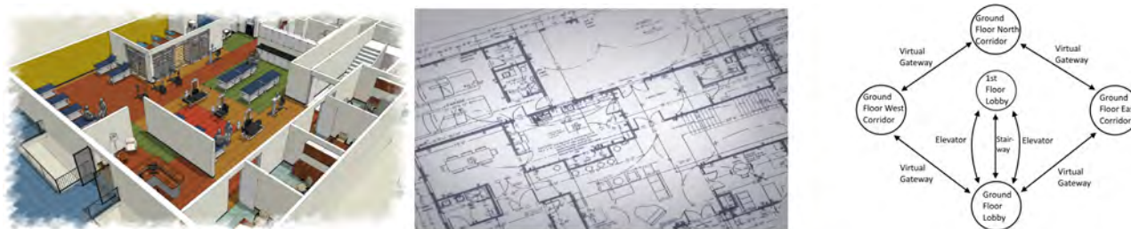
Figure 3. Example map views of complex office environments with gradual loss of details. left) Full 3D map view. middle) Floorplan in 2D. right) Topological view (Kun et al., 2017).
