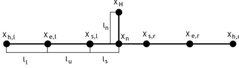
**Figure 1: The kinematics chain consists of the head  $X_H$ , neck  $X_n$  and, for each arm, a shoulder  $X_s$ , elbow  $X_e$  and hand  $X_h$ , which are at a calibrated distance  $l_u$  and  $l_l$ , the upper and lower arm lengths.**
