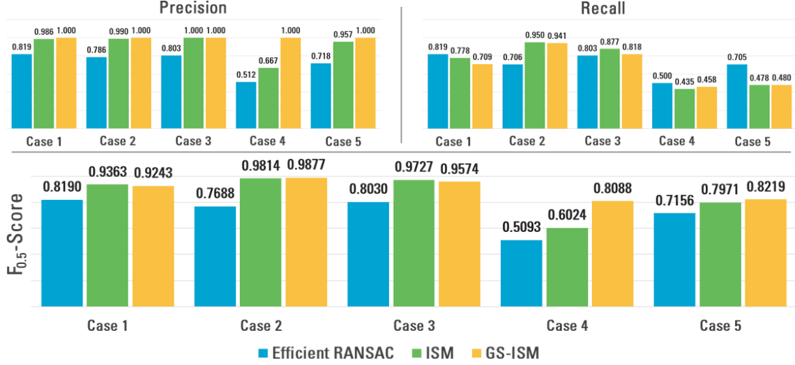
Figure 4. Comparison of precision, recall (top) and F_{0.5} -Score (bottom) between Efficient RANSAC [18], ISM [17] and our method.
