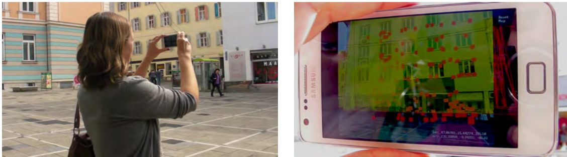
Fig. 1: From a SLAM map created on a smartphone ( left ), the system determines an accurate global device localization which can be used for augmented reality overlays ( right ). Here, a geo-registered city model is rendered in yellow on the building facade, with SLAM map points in red. The edges of the model are visibly aligned with the building extents.
