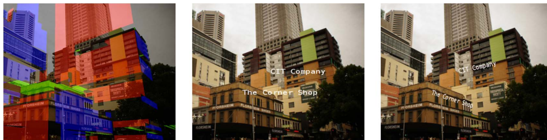
Fig. 13. Example of applying geometric constrains determined in real time from a single image. (Left) The computed surfaces and their orientation within the image. (Middle) The labels placed at their original position. (Right) Applying a layout algorithm based on geometric constrains such as the surface map and the edge map allows to automatically align the labels with their underlying geometry depicted in the current camera image.
