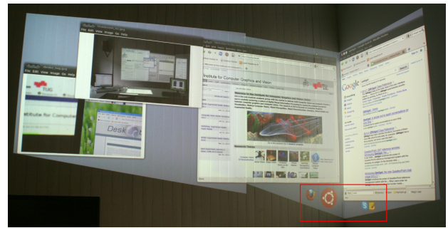
Figure 5: Desktop widgets on an irregular display are subject to semi-automatic window coordination and will therefore be gradually moved to peripheral areas where no larger items can be reasonably placed.
