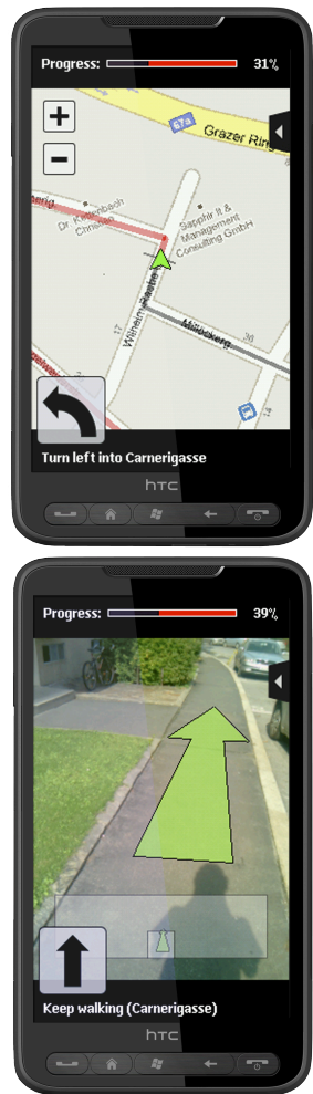
Figure 1. (Top) Tilting the phone down, users access the map, glyphs and text instructions. (Bottom) Tilting the phone up, users access an augmented view with arrows that provide egocentric navigational hints.
