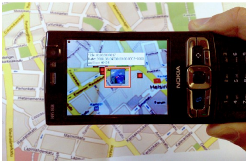
Figure 1. MapLens1 augments a paper map by superimposing registered icons and labels onto live video stream on the phone
