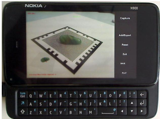
Figure 1. The Nokia N900 smartphone used for our evaluation. The screen depicts a scene from the modeling procedure. The current modeling result is rendered in the lower left corner.
