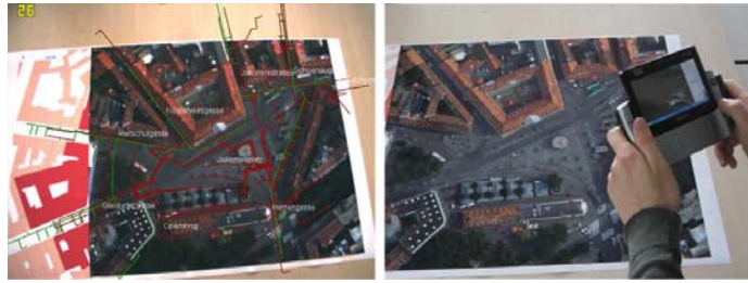
Figure 1: User is equipped with a mobile device that accurately renders 3D structures and information directly on top of the orthographic photo [4].
