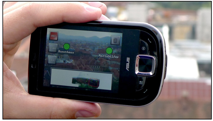
Figure 11. Running at 30Hz on mobile phones, our method gives room for end-user applications. Left: Our method can be used to guide users in taking hi-res photos of the environment to be later stitched with a desktop application. The system can show a live preview of where photos have been taken, to ensure optimal coverage of the whole panorama. Right: Our method can be used for annotating panoramas and sharing them with other mobile users coming later in-situ, or with desktop users.
