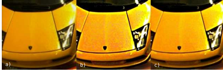
Fig. 4. Spatial coherence. This figure illustrates the problem arising from the emphasis of contrast in the focus area. A tungsten light on the metallic surface of this car model caused this particular artifact. Notice the red or green dust in the middle image. a) Original image. b) Image affected by naïve conspicuity enhancement. c) Image after applying our spatial coherence technique.
