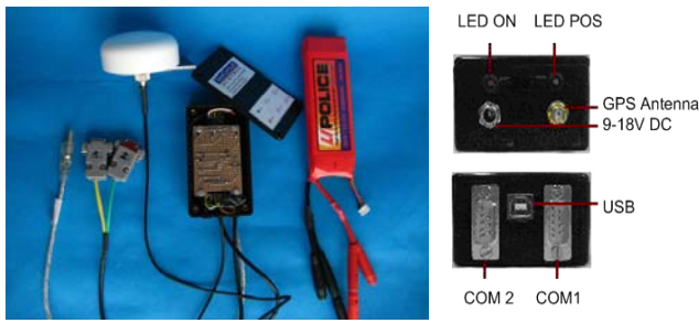
Figure 2: Novatel OEMV-1 receiver (DGPS/RTK) (11x6x3cm) placed in the middle of connectors, antenna and battery (left). Side view of the receiver (right).
