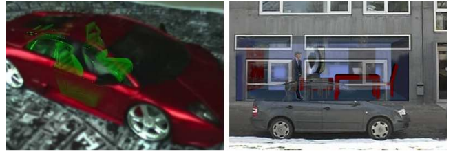
Figure 3: Final composed result examples. The resulting images of our technique preserve information of the occluder in order to aid for a better perception of spatial arrangements. (left) The seats and engine of the car can be seen through the car body. (right) The office inside the building can be seen through.
