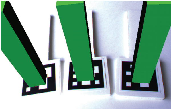
Fig. 12. Three markers with a low expected error. The error is calculated from the angle between the vector from the camera to the marker and the marker's normal.
