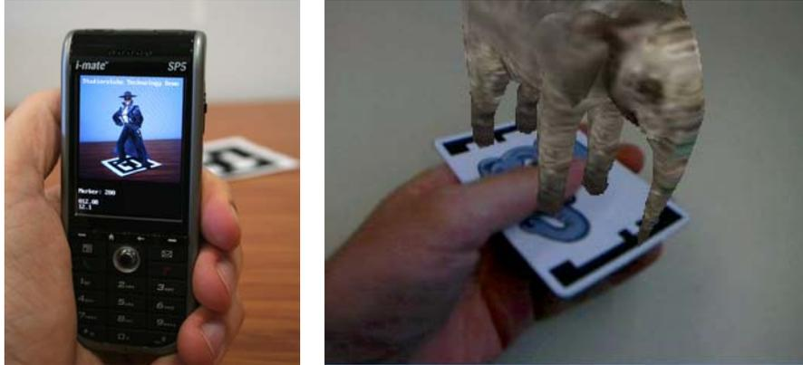
Figure 1. Examples of Augmented Reality on phones. Left: a virtual character on a square marker. Right: a virtual animal on a tracked playing card. In both cases the live camera feed is drawn as a video background and the virtual object is rendered on top of it.
