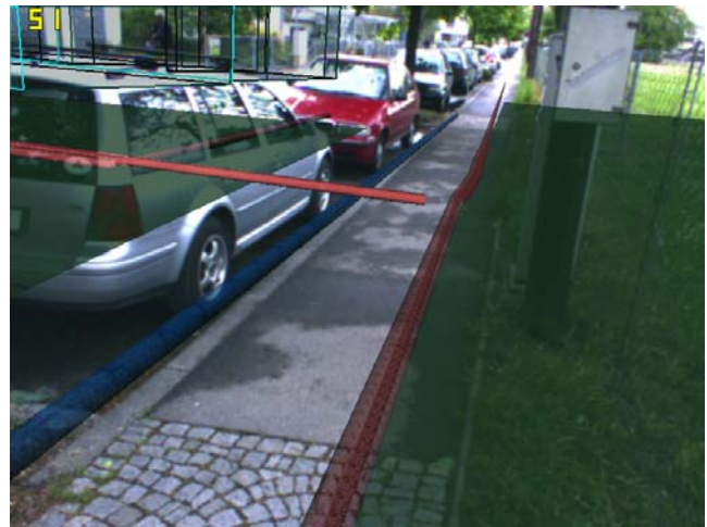
Figure 13: Land-register (cadastral) data superimposed on the real environment in employing AR visualization techniques.
