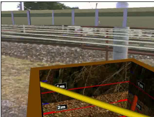
Figure 8: The excavation lens implements a virtual excavation in which the buried assets perceived in all three dimensions.
