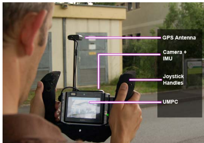
Figure 6: Vesp'R is a design for an ergonomic handheld Augmented Reality device designed around an ultra-mobile PC.
