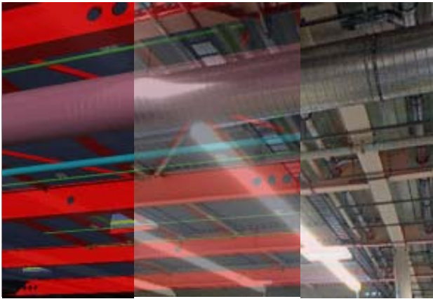
Figure 2. industrial environment with complex architecture and infrastructure; screen is split vertically into three segments: on the left pure virtual model, on the right pure photograph, AR overlay in between
