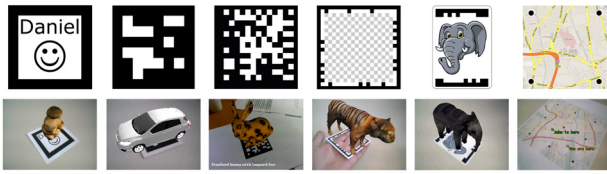
Figure 3: StbTracker supports a wide variety of markers: Template markers allow placing an image inside the rectangle; BCH markers directly encode 4096 IDs; DataMatrix markers can encode ~50 ASCII characters; Frame markers can have arbitrary or even no pattern at all; Split markers require only two bars on top and bottom, whereas the sides and content are free; Grid markers can span large areas of textured planar surfaces.
