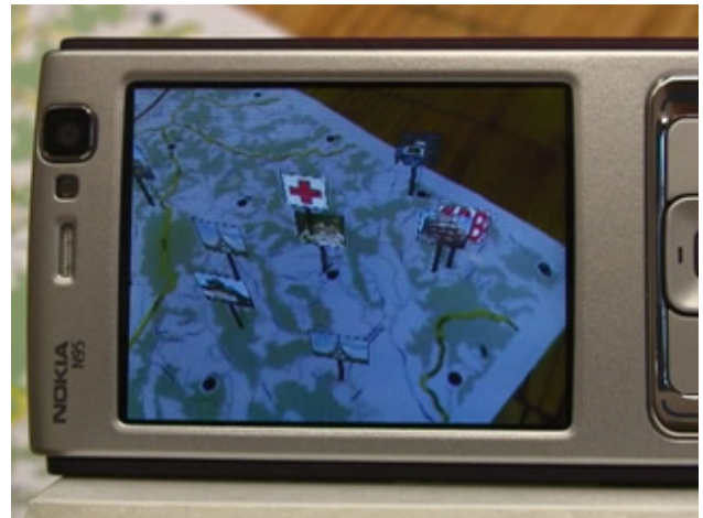
Figure 1: Nokia N95 running Studierstube ES superimposes geo-referenced content on a map of Graz
