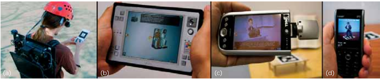
3 The evolution of mobile augmented reality hardware from (a) backpack systems to (b) Ultra-Mobile PCs, (c) personal digital assistants, and (d) smart phones.
