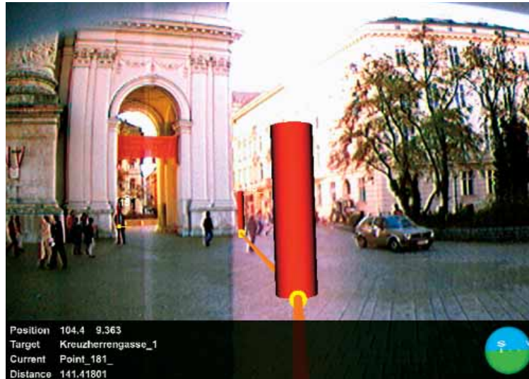
4 A visualization of the path to the selected target with clipping on known objects.
