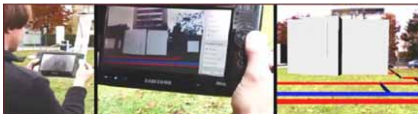
Figure 3: Tracked outdoor user seeing superimposed AR buildings and subsurface infrastructure (water mains, electricity lines in this example)
