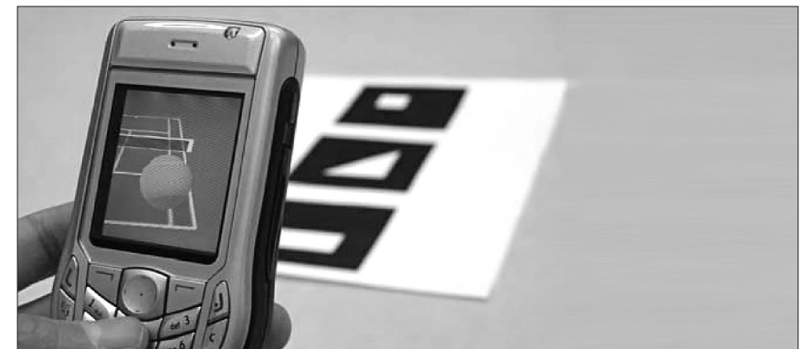
Fig. 12: AR Tennis [8], developed in 2005 at HIT Lab New Zealand also lets two players share a game of tennis but uses markers to establish a shared space for the players. The phone itself is used as a paddle to hit the ball, which requires a lot of physically movement with the device. Each phone can be fitted with a marker on the back so that it can be detected by the opponent’s phone for visual feedback.
