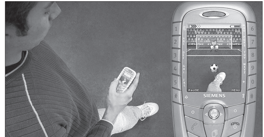
Fig. 9: AR Soccer [6] shows a virtual soccer goal and blends in the handheld's video image in the bottom half of the screen, letting a user view his own foot in the soccer environment. The aim of the game is to shot a virtual ball into a virtual goal. To do that, the player has to kick the ball with his foot, which is tracked using an advanced pixel flow detection algorithm. In contrast to simpler pixel flow methods such as used by the Mosquito Hunt game, ARSoccer accurately detects the edge of the moving foot and can thereby calculate the exact speed and direction of the foot hitting the ball.
