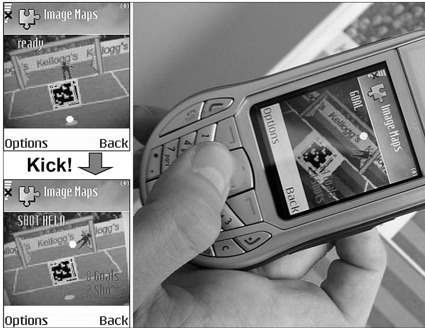
Fig. 4: Penalty Kick [12] is a simple example for a game of category (1). It uses a coarsely registered 3D marker, which can be printed on a poster or product package. The aim of the game is to shoot a soccer ball into a goal printed on the product package. The player can aim where to shoot the ball by rotating and tilting the phone. The virtual goal keeper will then try to hold the ball.
