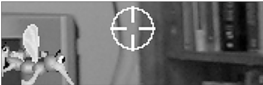
Fig. 5: Mosquito Hunt challenges the player to shoot mosquitos. The gun is pointed at the mosquitos by moving the phone in space. A simple pixel flow detection algorithm makes the mosquitos stay fixed relative to the environment. The world is captured by the built in camera acts as a backdrop for the game, while the mosquitos are rendered as 2D sprites on top of that background. The game only measures orientation, so that actually only the orientation of the device matters, while the position is irrelevant.
