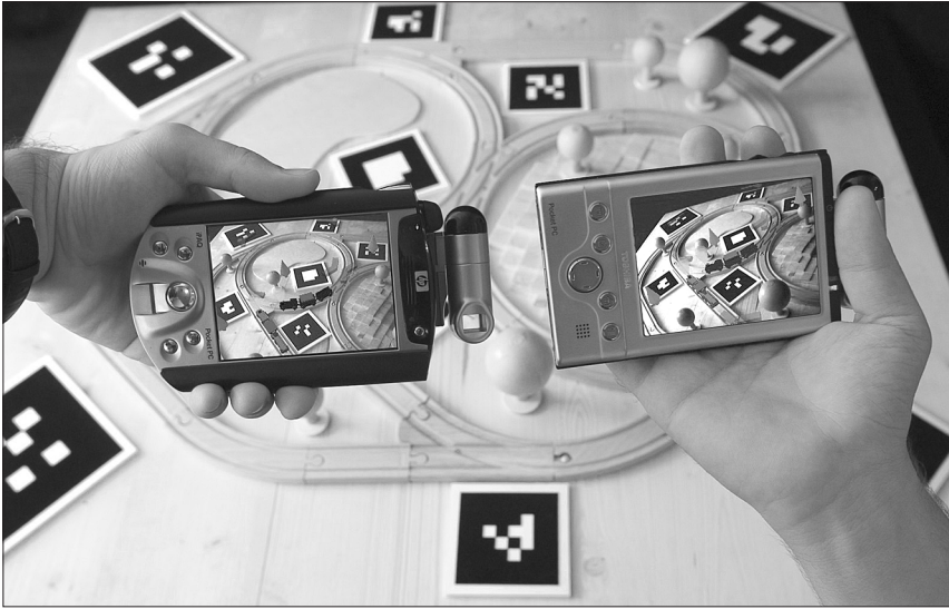
Fig. 2. Invisible Train is a collaborative game casting users in the role of engineers in control of virtual trains on a real wooden miniature railway track. Players can interact with the game environment by operating track switches and adjusting the speed of their virtual trains using the handheld's touchscreen. The current state of the game is synchronized between all participants via WiFi. The common goal of the game is to prevent the virtual trains from colliding. The touchscreen is very instrumental in operating the game, since it lets users select game elements such as junctions which are not in the center of the view. The game still requires a fair amount of physical movement, which has been reported to be an essential ingredient of the play value. However, the use of the touchscreen avoids excessive movements since users can overview and manipulate a sufficiently large part of the playfield at once.
