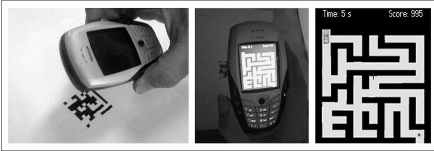
Fig. 6: Mobile Maze [5] goes one step further in the direction of pure VR by turning the handheld device into a purely simulated handheld maze game. The player has to guide a ball through a maze by tilting the physical maze itself. The software visually tracks the phone's orientation using a marker, but does not display any video image.
