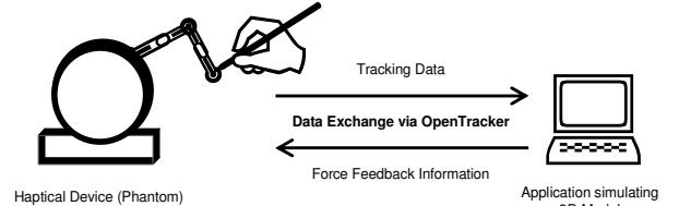
Fig. 8: Haptic device using OpenTracker data exchange
