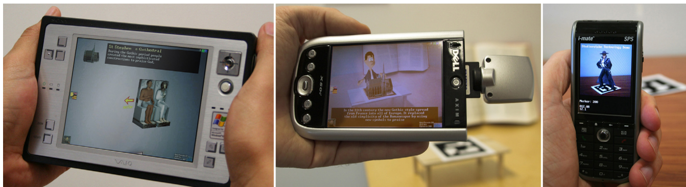
Figure 1: Devices for handheld Augmented Reality: UMPC, PDA and smartphone.
