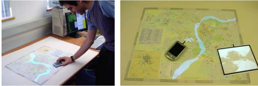
Abb. 1. (Left) a user interacting with an augmented map, (right) overview of the individual tools and example augmentation of the expanded river
