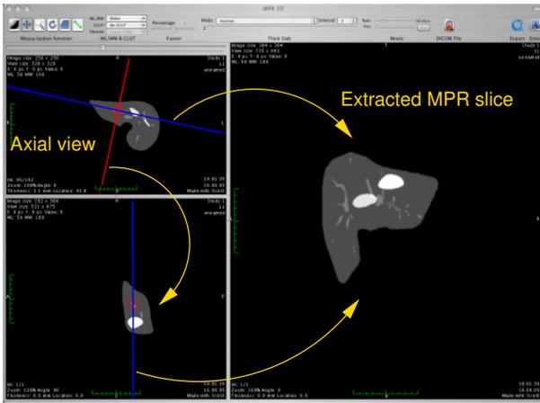
Figure 7: This screenshot shows a phantom medical dataset viewed in OsiriX using the 2D MPR technique. The upper left view displays an axial view from the top, the lower left view shows the interpolation of the upper red line, and the most right view shows the extracted slice of the blue lines specified in the previous views.
