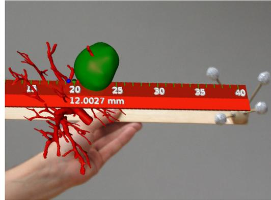
Figure 1: An additional props – the interactive ruler – can be used for measuring distances in a semi-automated way. The number displayed at the center of the ruler indicates the distances between two surface intersection points.
