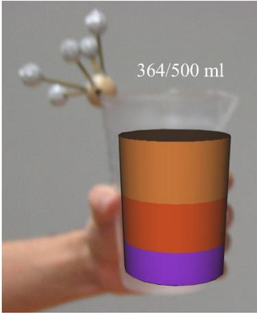
Figure 2: The measurement jug, shown as an overlay image, can be used as a volume calculator where volumes of individual objects are summed up. The overall measured volume is displayed numerically on top of the jug.
