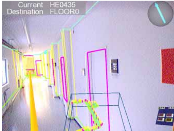
Fig. 7: Indoors, a combination of directional arrows, highlighting of exit, compass (upper right) and world-in-miniature (lower middle) is used to help a user navigate the environment.
