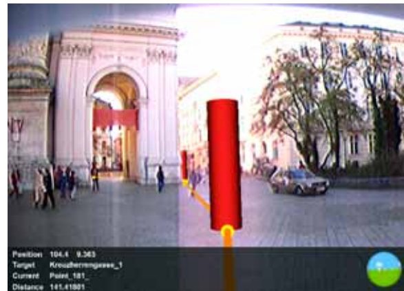
Fig. 5: An outdoor navigation guide for a pedestrian visualizes the selected route as a series of waypoints. Note the correct occlusion between the route and the archway.
