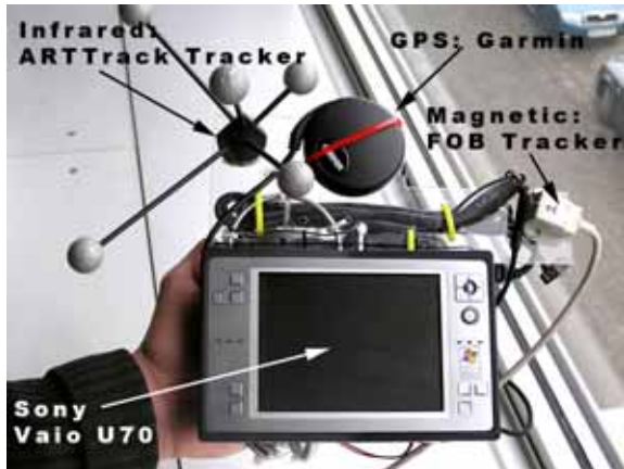
Fig. 2: This handheld AR platform is based on a mini tablet PC that is operated as a video-see through "magic lens" device. It currently supports five different tracking technologies (3 shown) and weighs less than 1.5kg.
