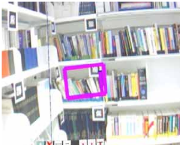
Fig. 8: The “Augmented Library” allows a user to quickly locate the shelf on which a book of interest can be found, by emphasizing the relevant location.
