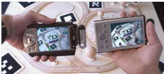
Fig. 3: The smallest fully featured AR platform to date is based on commercial PocketPC 2003 handheld computers. Using an embedded camera, these devices can perform optical marker tracking and real-time 3D graphics at ~20fps. Shown is the "Invisible Train" multi-user game successfully demonstrated at SIGGRAPH 2004.
