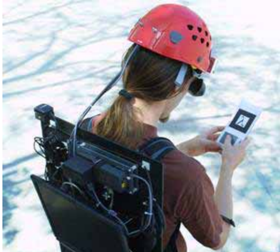
Fig. 1: The backpack system is based on a conventional notebook computer displaying stereoscopic graphics overlays in an optical see-through head mounted display.
