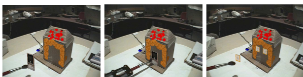
Figure 9: Interactive placement of labels: Left and middle – placement of a virtual door on a real house; right - placement of a window with the “label and copy” tool.
