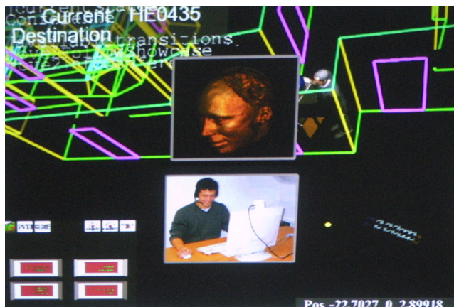
Figure 9. An indoor tour guide application, running on the desktop developer setup. A world-in-miniature view on the model of the building is shown in the background, and location-dependent HUD overlay graphics is presented to the user as she roams the building.
