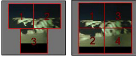
Fig. 7: Schematic view of the two and three projector arrangements.
