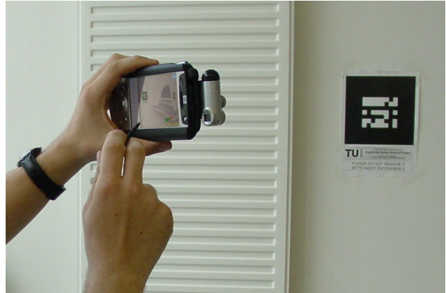
Figure 1. The self-contained handheld AR system can track optical markers in real time.
