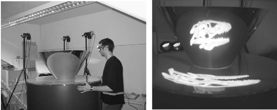
Fig. 1. A head-tracked user (left) observes a warped image (right) inside the Virtual Showcase.
