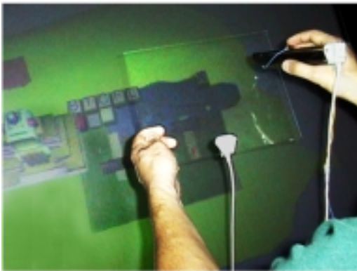
Figure 1: The transparent PIP and pen props (taken from [21]).
