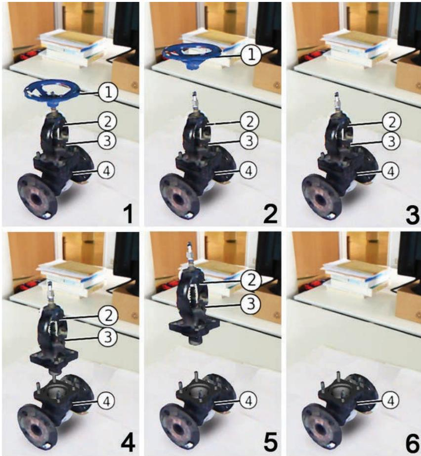
**Figure 1.17** Automatically generated disassembly sequence of a valve. Courtesy of Peter Mohr.
