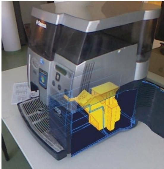
**Figure 1.16** Ghost visualization revealing the interior of a coffee machine to guide end-user maintenance. Courtesy of Peter Mohr.
