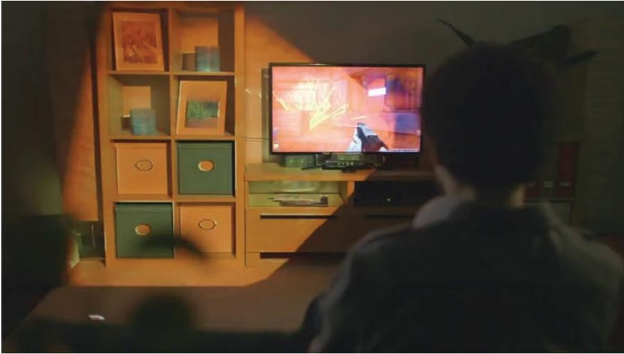
**Figure 1.29** Using a TV-plus-projector setup, the *IllumiRoom* extends the game world beyond the boundaries of the screen. Courtesy of Microsoft Research.
