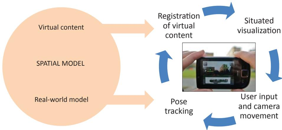
**Figure 1.1** AR uses a feedback loop between human user and computer system. The user observes the AR display and controls the viewpoint. The system tracks the user's viewpoint, registers the pose in the real world with the virtual content, and presents situated visualizations.
