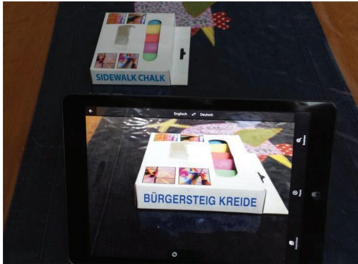
**Figure 1.21** Google Translate superimposes spontaneous translations of text, recognized in real time, over the camera image.
