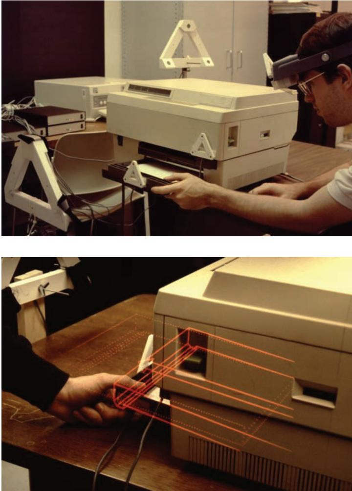
**Figure 1.4** (top) KARMA was the first knowledge-driven AR application. (bottom) A user with an HMD could see instructions on printer maintenance. Courtesy of Steve Feiner, Blair MacIntyre, and Doreé Seligmann, Columbia University.
