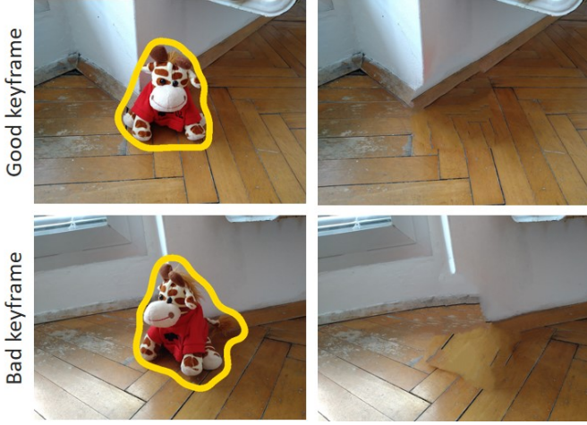
Fig. 7. “Avoid depth discontinuities” (rule 5) The top and bottom rows show good and bad keyframes according to rule 5. A large depth discontinuity wrongly connects the wall edges. The far wall on the left gnaws into the front wall on the right.
