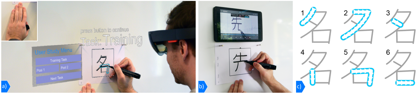
Figure 7. Retargeted Kanji tutorial and final revision of AR visualization. (a) The AR visualization is presented using an Optical See-Through HMD (Microsoft HoloLens) and a handheld clicker that the user is holding in one hand. (b) The video tutorial is shown on a tablet mounted right above the drawing area. This reduced the influence of head motion. (c) Our final glyph design encodes the direction of the stroke on its border using arrow heads. The system presents one glyph at a time next to a full preview of the final drawing. This picture shows the six instructions presented to the user in AR.
