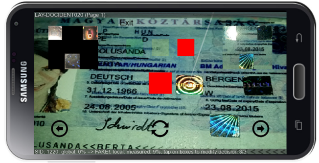
Figure 5: Summary of image capture presented to the user. Reference information is shown left, obeying the layout of sub-elements, while the best match is shown on the right hand side along with local and global ratings of the system indicated as colored squares.
