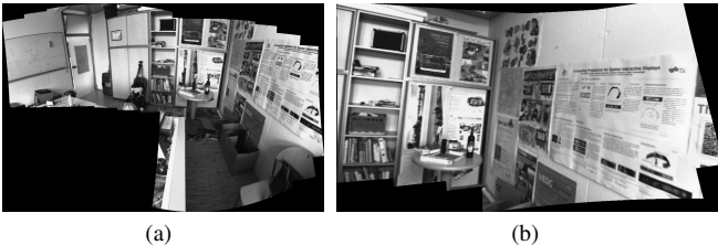
Figure 6: Panoramas generated from keyframes of two local panorama maps. The local panorama map (a) was created in the period during frame 800 and 1200. The local panorama map (b) was created in the period during frame 1500 and 1800. Both panoramas depict the scene from two different view points with sufficient parallax for triangulation (e.g. the wall on the right-hand side).
