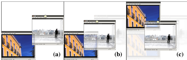
Figure 6. Semi-automatic window layout: (a-b) the user drags a window towards the left, which causes an overlap with another window. The window layout persists as long as the amount of covered information is low. (c) If more information is occluded, the obscured window is re-positioned to leave the most important window content uncovered. Window trails were added for illustration purposes.
