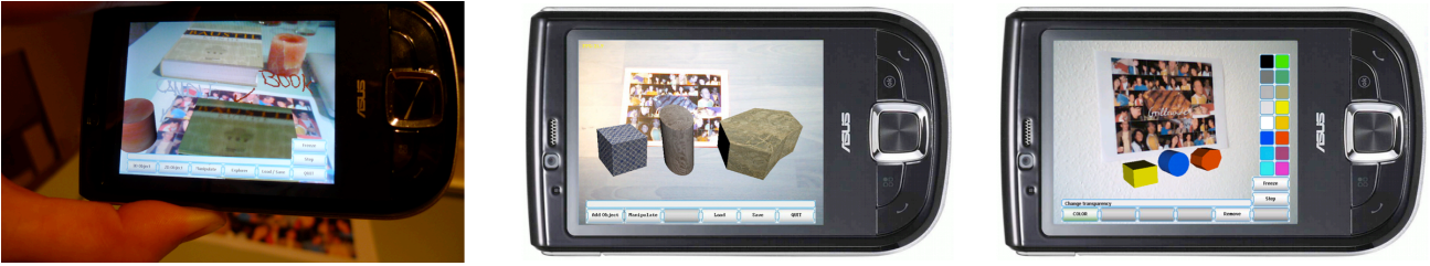
Figure 3: Example showing created augmented 3D content and interface using the system configured for small working environments, Left: Augmented scene with augmented duplicates of real objects (book and candle) , Middle: Augmented scene showing different object shapes with different applied textures, Right: Augmented scene showing different objects with different colors and interface for selecting colors.
