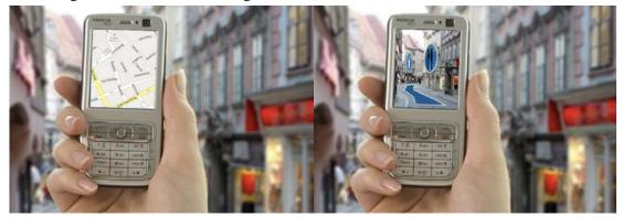
Figure 1: Contrary to traditional map displays (left), AR 2.0 will navigation information on top of the images captured by mobile phones (right). Users will also be able to create and update 3D registered content, creating a location-based social network.
