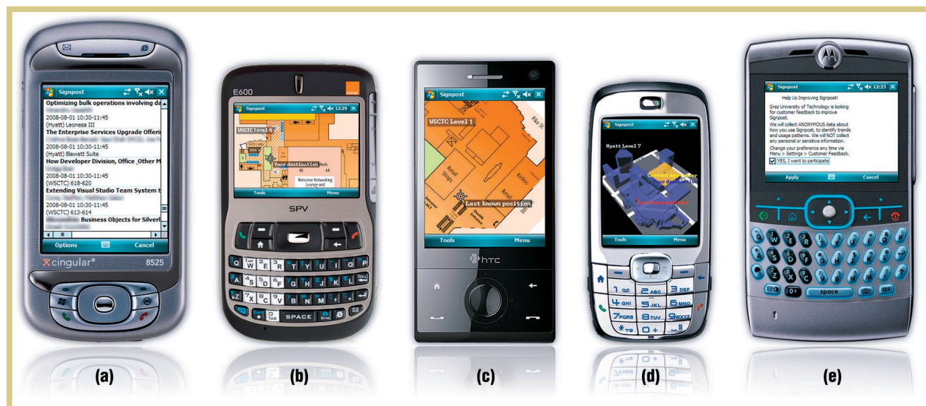
Figure 3. Examples of phones running Signpost and screenshots of the application: (a) HTC Cingular 8525, (b) Orange SPV E600, (c) HTC Touch Diamond, (d) HTC S710, and (e) Motorola Q. Signpost supports various form factors and resolutions of the screen, and different input capabilities (both keypad- and touch-based).
