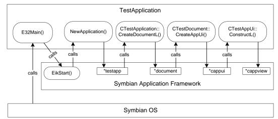
Figure 10. Sequence of initializing up a Symbian application
